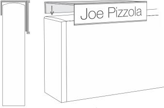
The custom bracket can be made to attach via the groove in the screen cap.
