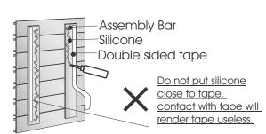
REAR VIEW - With Assembly Bars. (Signs from 147mm & up in height)
